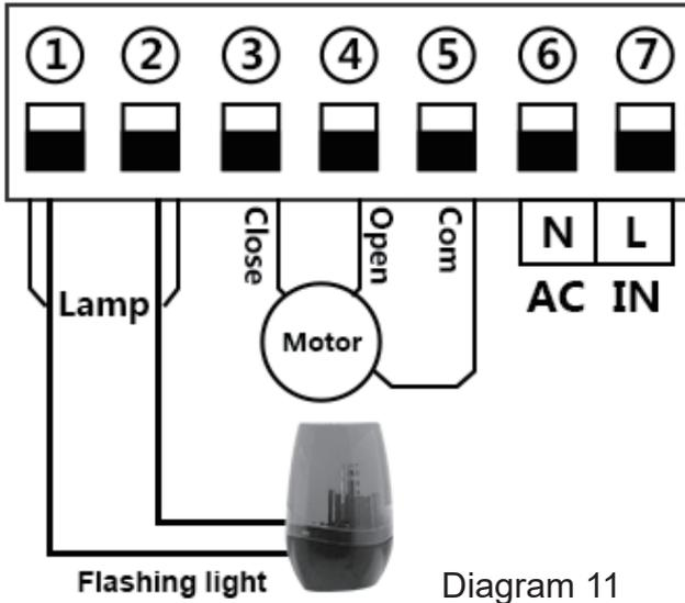
Terminal ① and ② is for connecting with the flash lamp .
