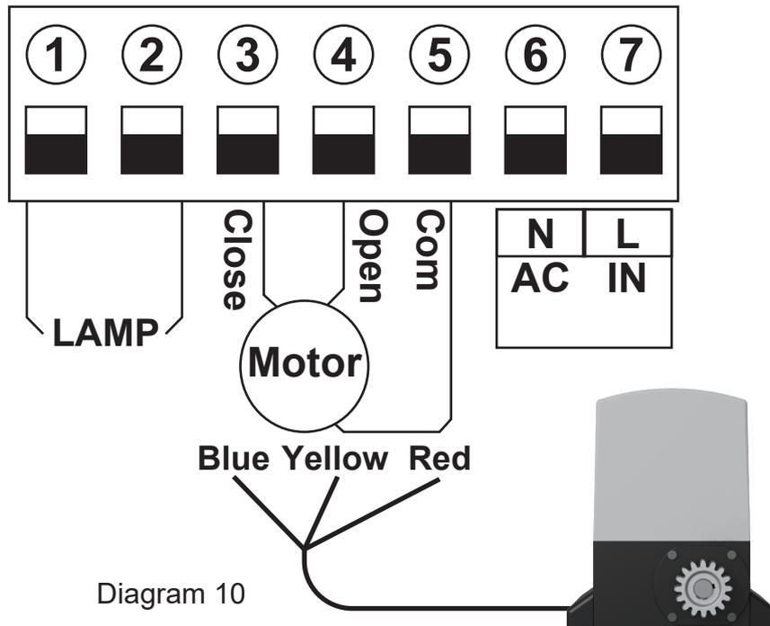
Terminal ③, ④ determines the forward and backward direction of the motor
