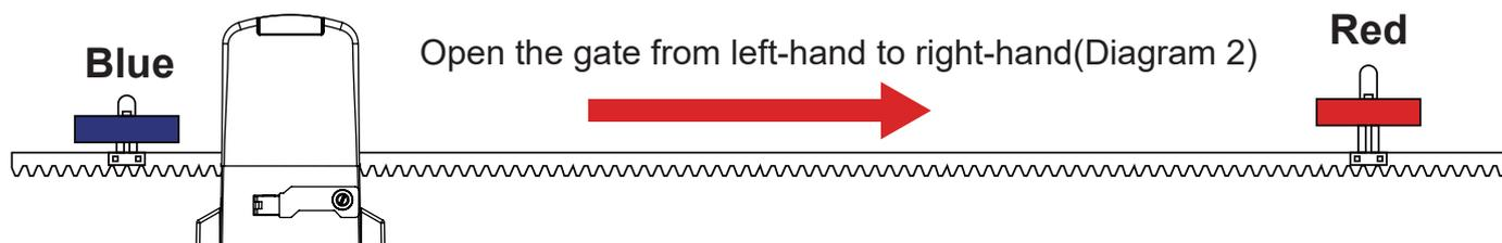
If you install the motor on the left of the gate, please adjust the blue and red limit magnet position as below picture show.
