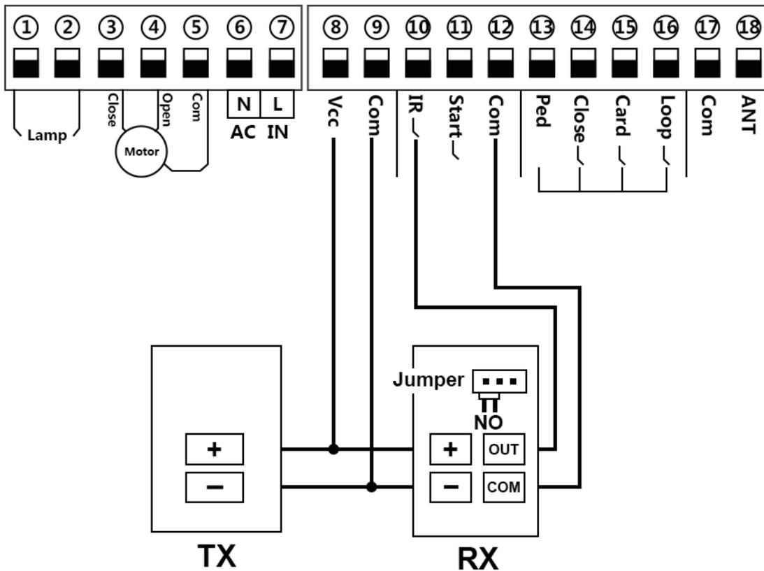
Connect terminal ⑫, with the “ COM ” of photocell RX.
